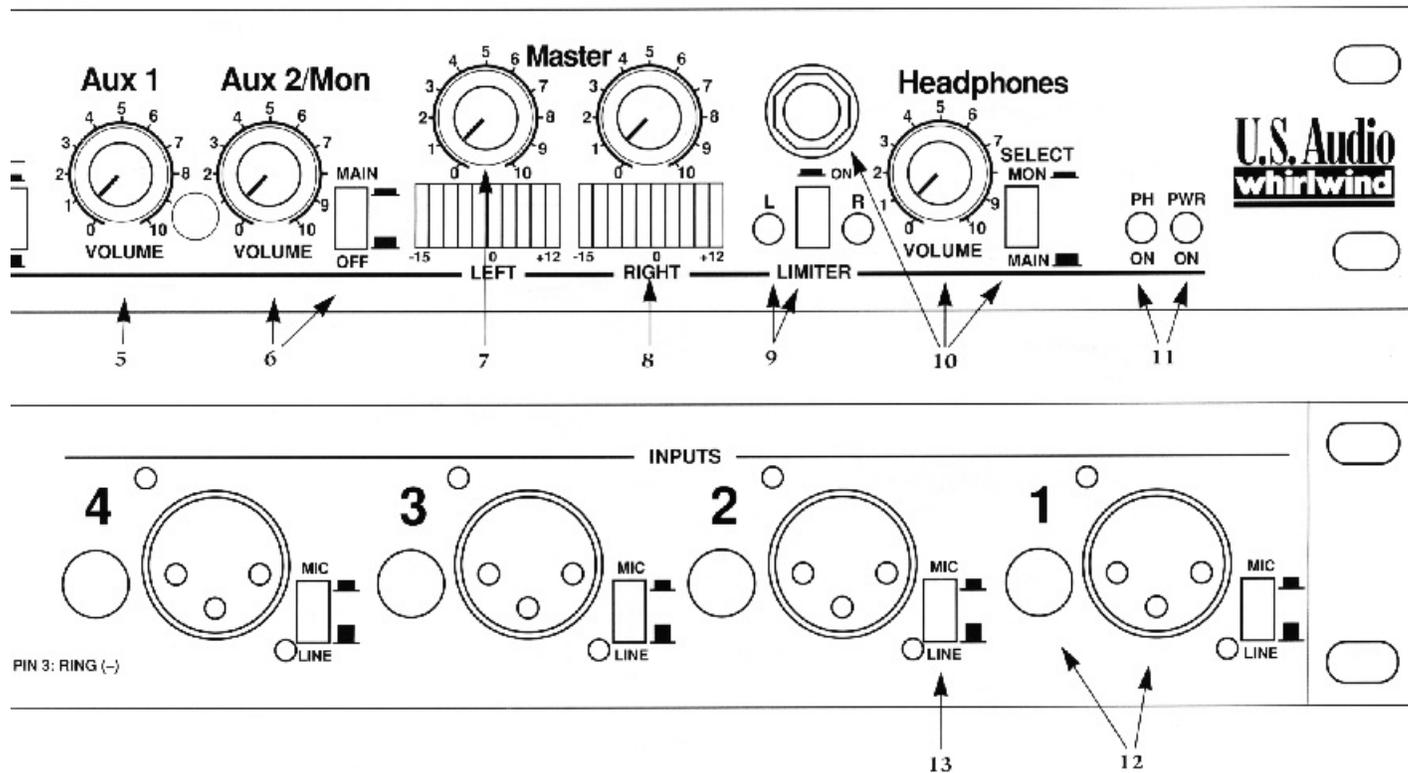
**12. Input 1/4 TRS and XLR Jacks** are AC coupled through phantom blocking capacitors with pin 2 being positive wired to tip, pin 3 being negative wired to ring and pin 1 being common wired to sleeve.
